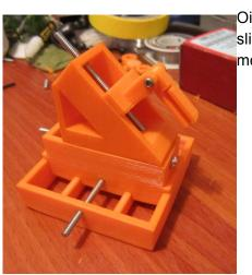
Oil the bottom of the Z-axis and insert into y-axis. Part should slide back and forth easily, especially after you "break it in" by moving the piece rapidly back and forth.
