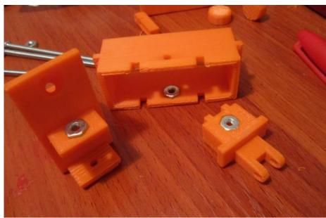
After the glue dries, remove screws that were helping to set nuts. Add some machine oil to nut threads
