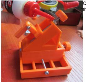
Oil! Oil ALL Points on each axis. Oil the point between the nut and the wall....
