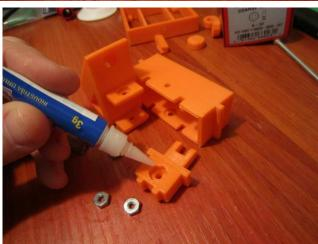
Add a couple dabs of super glue to the Hexnut inset walls. Avoid getting glue inside the inner hole. Place Hex-nut inside, sanded side down
