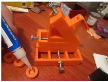
Now it's time for the knobs. Add a bit of superglue to the inside of the knobs.
