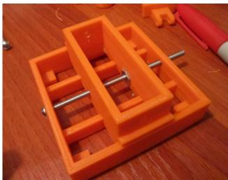
Screw in 3.25 inch fastener. Screw in all the way so that there is no space between the head of the screw and the outer wall.
