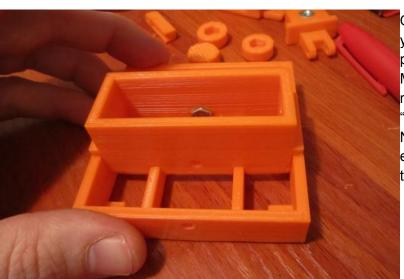
Oil all touching edges, and place y-axis inside x-axis. With oil the part should slide back and forth. Move back and forth the part rapidly with elbow grease to "break in" part. YOU SHOULD NOT NEED TO SAND PARTS to enable a fit. Move back and forth to "break in"
