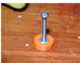
As you have done in previous steps, keep nut aligned in hole during glue drying step by screwing in fastener.
