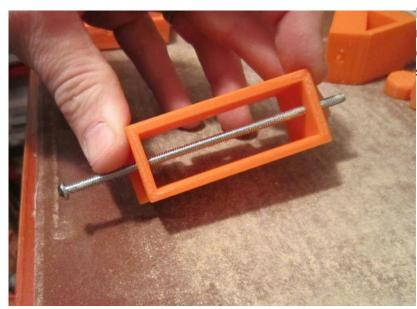
Ream the Y-axis. Note, only ream along the long dimension (as in picture)...NOT in the short dimension
