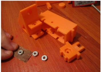
Now it's time to glue the three 6/32 Hex-Nuts to the moving pieces. Lightly sand one side of each nut.
