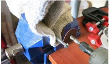
2. Cut the 4 inch faster down to 3.75 inches, FROM THE HEAD end. A sock or cloth around fastener while it is in the vise will reduce damage to threads.
