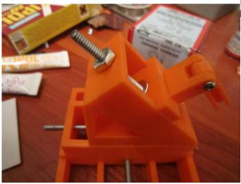
Hand tighten HEX nut on fastener. Tighten by hand to 2-3 finger force strength
