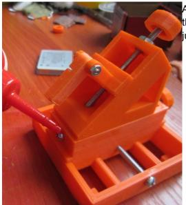
Also apply oil along the head of the screw. Repeat for the other 2 axis. Also oil all plastic/plastic sliding junctions.
