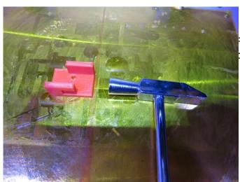
Run hammer along table and tap lower end of piece (Not the walls)
