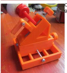
Oil the point where the nut is on the moving part, and in general along the fastener...
