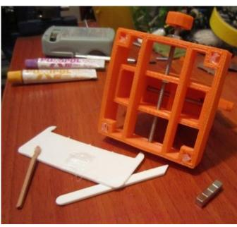
Now it's time for the magnets. Prepare some more epoxy, and place liberally in the holes in the base. Do not let epoxy spill out of hole though.
