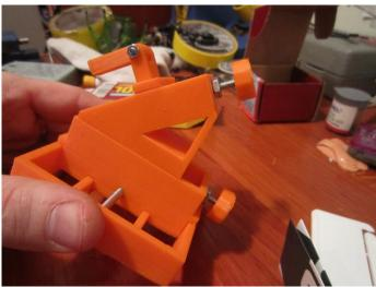
Install Knobs. Make sure the knobs look straight when viewed from the side and are not crooked. If knob appears not to fit, use elbow grease. Some knobs will fit better than others. This is due to the limitations of the 3D printer and cooling of the plastic.
