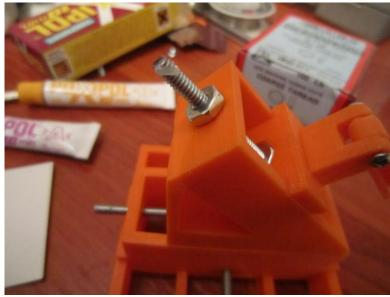
Apply some epoxy to end of the fastener
