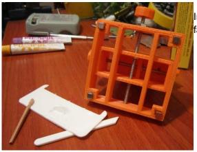
Insert Magnets. Try to do with magnet poles all facing same direction.
