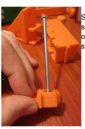
Screw in 3 inch fastener to secure nut and keep it straight while it the superglue dries. Screw in fastener all the way down, but not sticking out. **MAKE SURE FASTENER IS STRAIGHT**. This is critical for smooth operation of the moving part and diminishes wobble.
