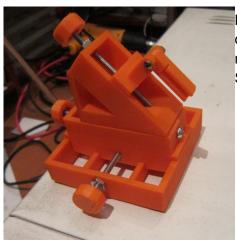
Magnets need to be leveled now. For this, use a flat piece of metal. Place the Searcher on the metal in a quick, rapid motion, so that magnets do not pull out of base. Leave Searcher alone for 1-2 hours for epoxy to set.
