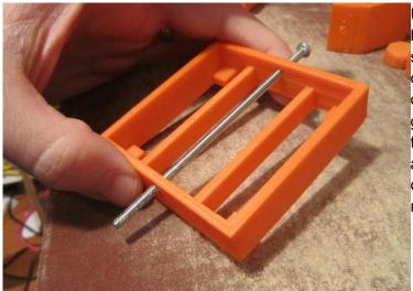
Using the 4 inch screw, "Ream" the holes in the X-axis so that the screw slides back and forth with ease. This is critically important for smoothness of operation. This may take a little elbow grease, as the hole is slightly smaller than the screw, and reaming removes a small layer of plastic from the inner diameter. This is by design so that the reaming makes a tight fit.
