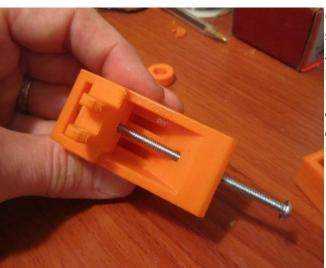
Oil the Electrode holder #1, and make sure it slides back and forth. Move back and forth to "break in." This is a very tight fit by design. Only sand if absolutely necessary. Make sure the side of the electrode holder WITHOUT the nut is facing down. Screw in 2.25 fastener from the bottom.
