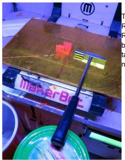
The small pieces can be very hard to remove from Replicator table that had an an acetone slurry applied. Removing by hand with force often damages the parts. I bought a small rock/hobby hammer, and a forceful, smart tap on side will liberate pieces. This doesn't result in noticable blemishes on piece but you should check.
