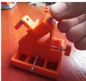
Now it's time to "break" the light bond that has formed between the nuts and the plastic. Use a quick, forceful turn of each knob. The nut should stay affixed in place to the fastener, and thus turning the knobs causes the moving parts to begin sliding on their axis. It will seem rough, so you need...
