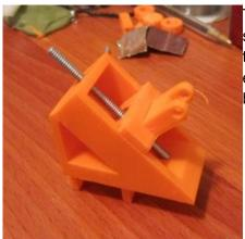
This is what it should look like. Make sure head of fastener is screwed in from underside is as far in as it can go. A way to test this is to keep turning with a screwdriver when you encounter resistance. The electrode holder #1 should then begin to move.
