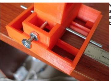
When installing the base axis, use a ruler and measure both sides to ensure the same length of the bolt is sticking out of both sides -- it should be ~3/6 inches
