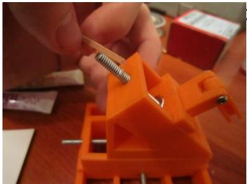
Apply a small bit of epoxy 1/2 inch above where fastener comes out of z-axis.
