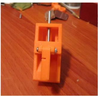
Insert electrode holder #2 in electrode holder #1, and secure with the ⅓ inch long 2-56 fastener and accompanying nut.
